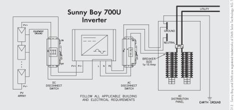
inverter's IGBT power stage generates a nearly perfect sine wave with the lowest harmonic distortion in the industry and meets ultra-strict FCC EMC standards. SMA's unique string inverter technology makes future system expansion simple. SMA advanced communication options are available to satisfy almost any application.
